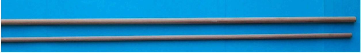
(a) cross grains make for a weakened mast
